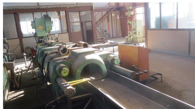
4- Hydraulic press, horizontal, 600 tons
