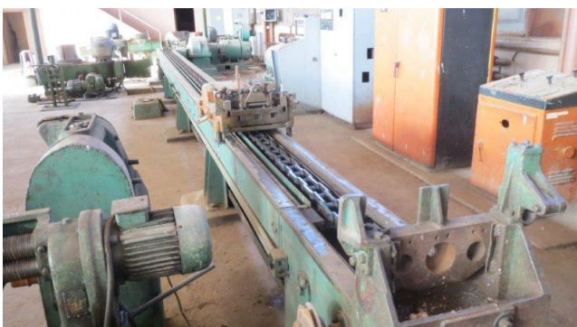
5 - Towing machine for wire up to \phi = 4 mm
