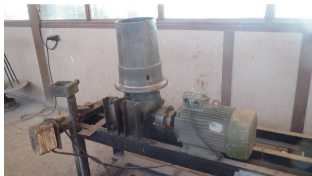
6 - Towing machine for wire up to \phi = 2 - 8 mm
